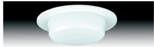
MODEL NO: RT-4-CF-ST-DL-1-13W-VL DESCRIPTION: DROP GLASS LENS SHOWER TRIM SIZE: 4-7/8" DIA LAMP/WATTAGE: 1 x 13W QUAD LAMP
