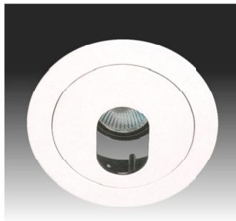
MODEL NO: RT-4-LV-SA-WH-50W DESCRIPTION: 4" LOW VOLT. SLOT APERTURE WHITE W/BLACK INSERTER SIZE: 4-7/8" DIA LAMP/WATTAGE: 12V MR-16/50W MAX
