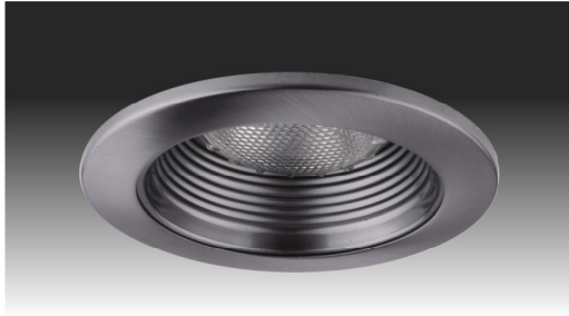
MODEL NO: RT-4-CHR-50W DESCRIPTION: 4" LINE VOLT.NATURAL CHROME BAFFLE SIZE: 4-7/8" DIA LAMP/WATTAGE:50W MAX.R20/PAR20
