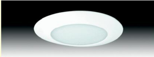
MODEL NO: RT-6-CF-ST-AL-1/2-13W-VL DESCRIPTION:ALBALITE SHOWER TRIM SIZE: 7-1/8"DIA LAMP/WATTAGE:1 x 13W OR 2 x 13W QUAD LAMP
