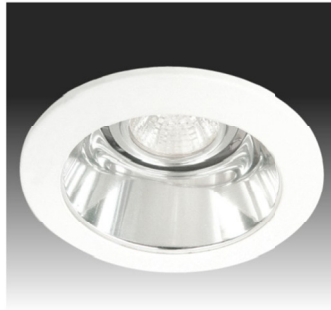
MODEL NO: RT-4-LV-CR-50W DESCRIPTION: 4" LOW VOLT. CLEAR REFLECTOR W/CLEAR INNER RING & WHITE OUTER RING SIZE: 4-7/8" DIA LAMP/WATTAGE: 12V MR-16/50W MAX
